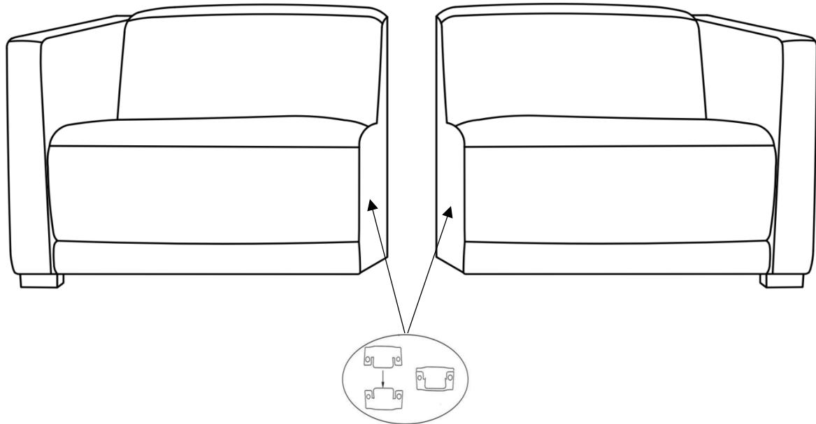
Connect the two sections by lifting one section slightly and aligning the connectors.
