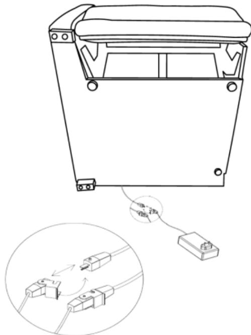
Attach the power source securely. Make sure to close the clip lock to prevent the connection from coming loose during use.
